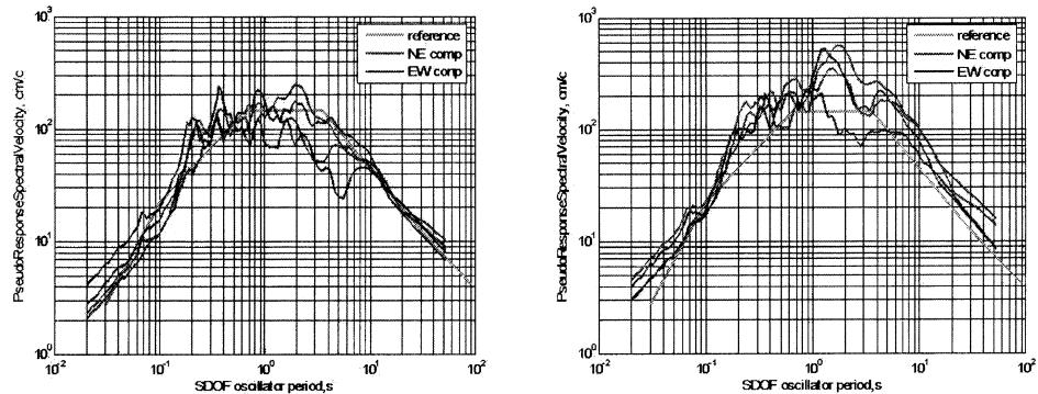
**FIGURE 4.** PSV Response spectra for horizontal components only, both piers on one plot. variants 222 (left) and 224(right)
