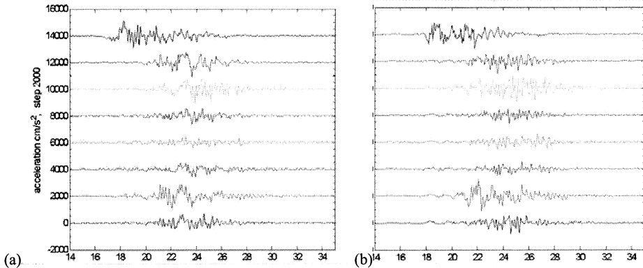
**FIGURE 7.** Eight sample functions of the ground acceleration at Torre Sicilia for the horizontal components: (a) NS and (b) EW. Vertical interval between zero-lines of traces is  $2000 \text{ cm/s}^2$ . The first trace is for the less usual source sample function, when a large asperity happened to coincide with the spot with the highest permitted propagation velocity.
