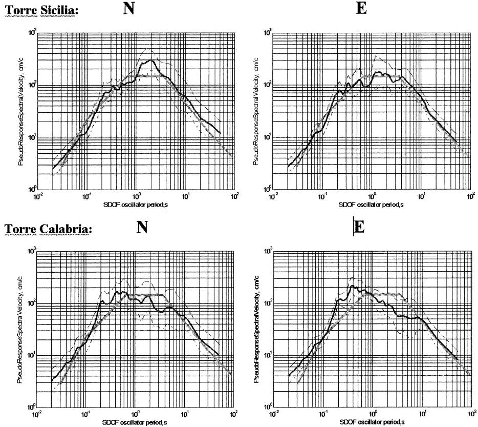
**FIGURE 6** .Median, and +/- 1 r.m.s. deviation corridor, for PRV for two horizontal components and the two piers.
