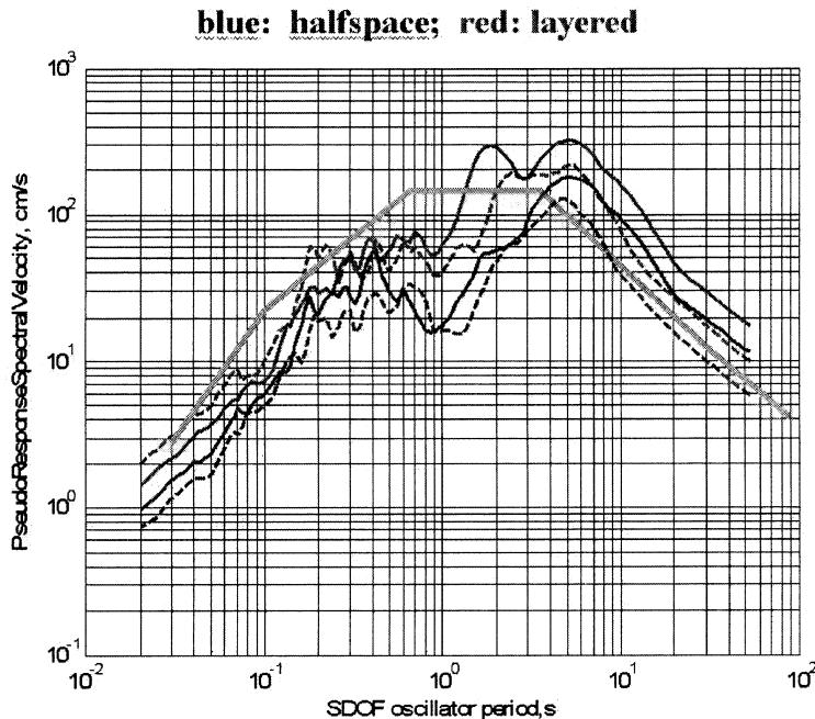
**FIGURE 8.** Effect of a layered crustal model against the case of a half-space with average-crust properties. Case of Torre Sicilia pier, solid line component NS , dashes - component EW, blue: halfspace; red: layered. The strongest resonance is at  $1.5-2 \text{ s}$  period, it makes amplification as high as 4-5 times with respect to the average crust. With respect to the “engineering hard rock”, such an effect will be significantly reduced.
