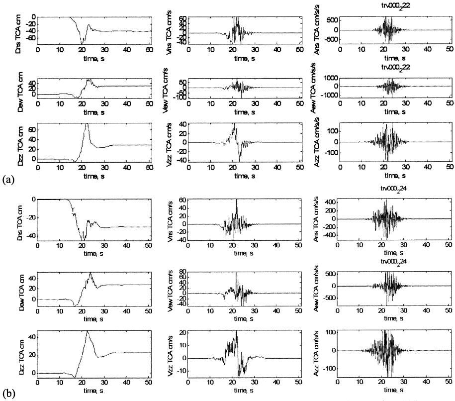
**FIGURE 3.** Ground motion at pier Torre Calabria: (a): variant 222, (b) – variant 224; in each block, from left to right: displacement, velocity and acceleration; from top to bottom: NS, EW and Z component.
