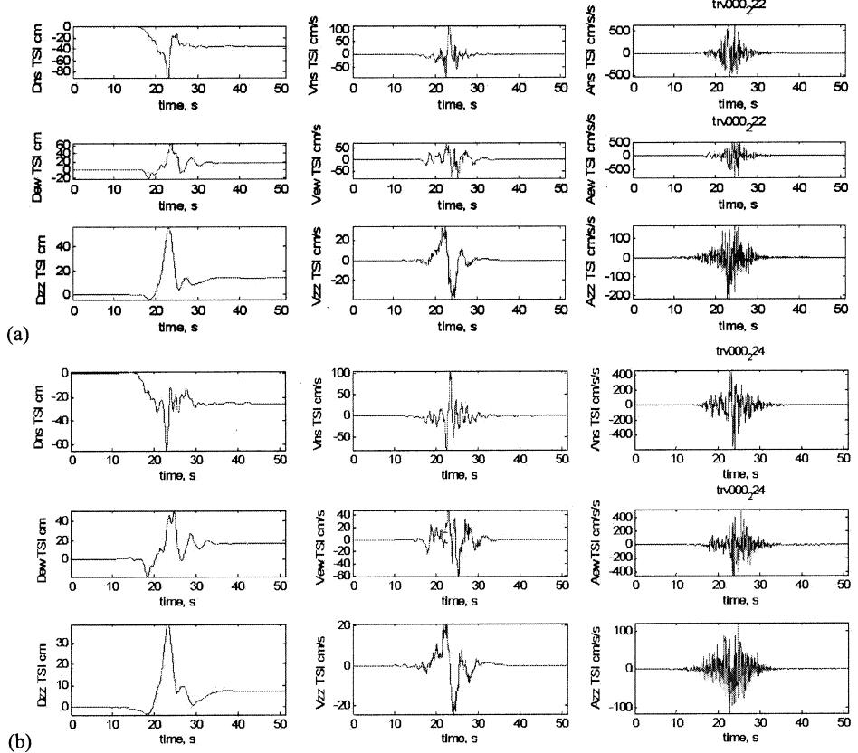
**FIGURE 2.** Ground motion at pier Torre Sicilia: a) – variant 222, b) – variant 224; in each block, from left to right: displacement, velocity and acceleration; from top to bottom: NS, EW and Z component.
